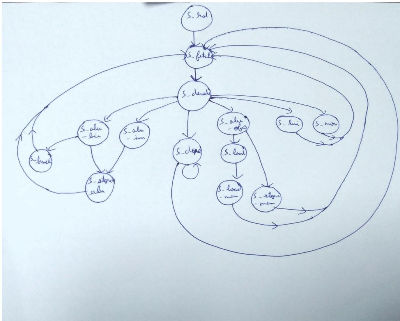
FSM of the controller is expressed in the VHDL process below with the states shown in above diagram
